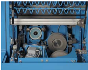
Edge finish module for operating side and base edges
