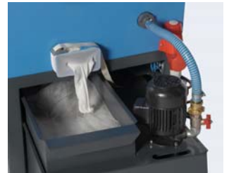
Residue-free grinding fluid through filter socket system
