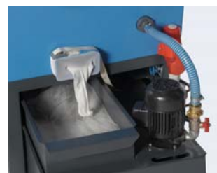
Residue-free grinding fluid through filter socket system
