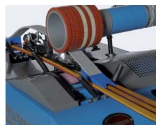
Exact stone structure grinding over the entire length
