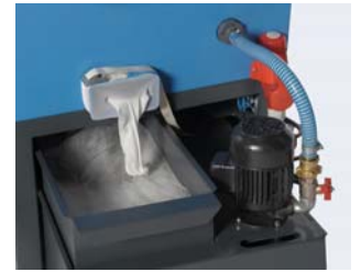
Residue-free grinding fluid through filter socket system
